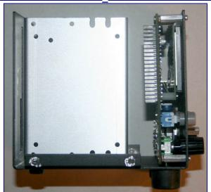
STEP 3: Attach the SR-Base standoffs to the sub-chassis
