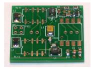
**STEP 9: Install the attenuator relays RLY1 and RLY2**
