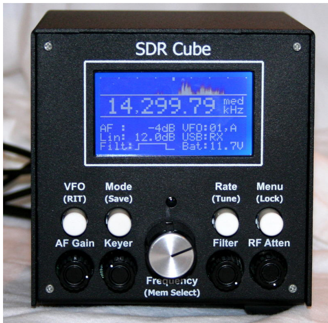
Figure 1: The SDR Cube Transceiver is dimensioned at 4" x 4" x 4", containing a full user interface, DSP processing, I/O connectors on the rear panel, and 27 in 3 shielded space internally for Softrock.
