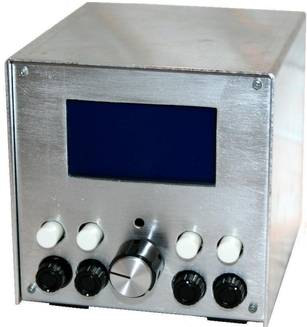
Photo 1: Cube prototype prior to application of black powder coating and white silkscreen labeling. Designed as initial companion to NUE-PSK digital modem, future growth will encompass modem functions and more.
