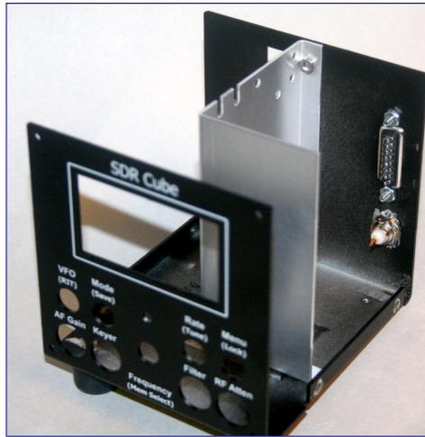
[ ] **STEP 6:** Attach the smaller rubber feet in the rear, and the larger rubber feet in the front of the chassis bottom. This arrangement will allow the SDR Cube enclosure to tip up from the table surface for the operator to more easily use the controls and see the LCD.
